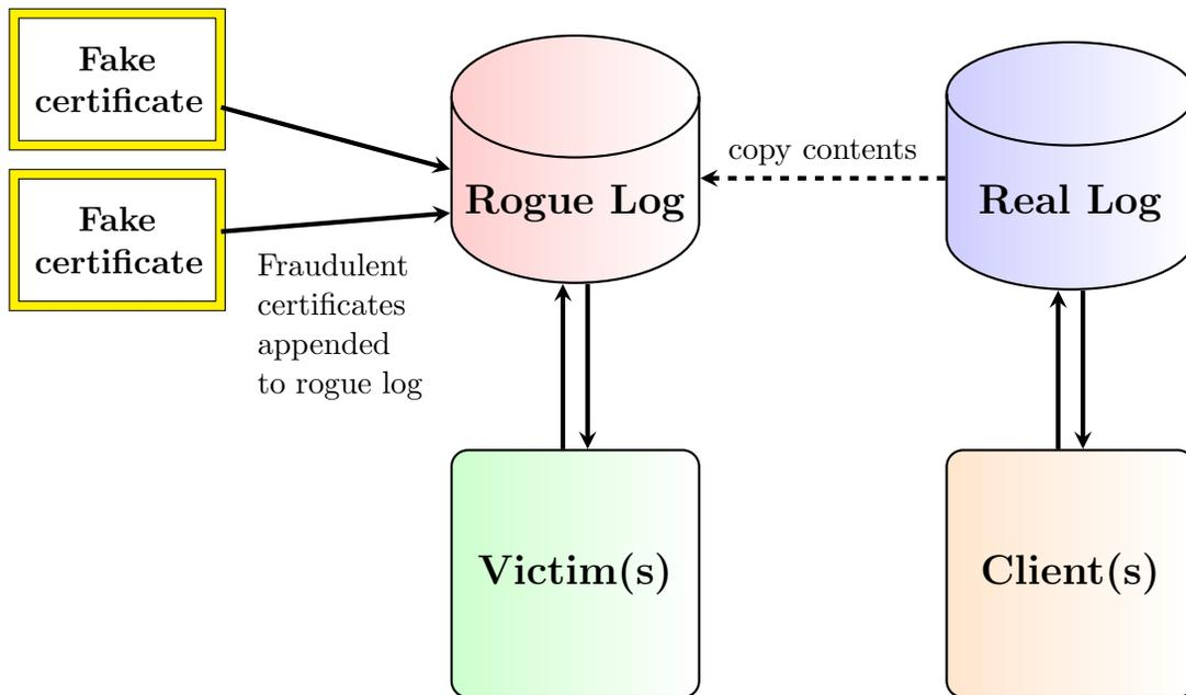
Figure 3.5: An Illustration of a split-world attack. The attacker copies the entire contents of a log and modifies it to include fraudulent certificates, presenting this rogue log to a set of isolated victims who have no means to verify consistency.
