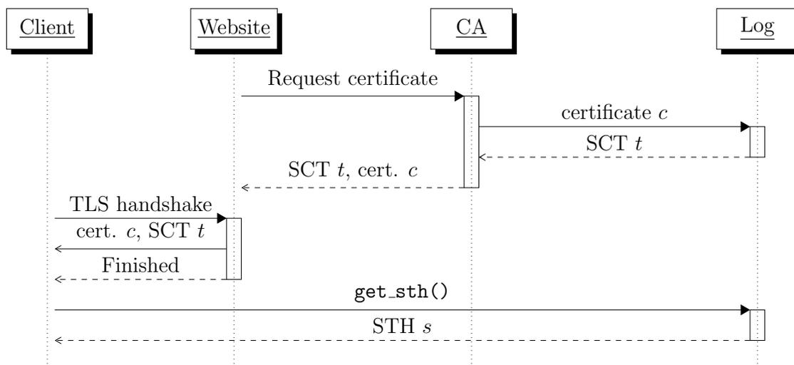
Figure 3.2: Communication flow of CT between a website, certificate authority (CA), log server and client. Anyone is capable of asking for a signed tree head (STH) at any time which contains up-to-date information about the log. In this figure, we assume that X.509 extensions are being used to deliver signed certificate timestamps (SCTs) with the certificates.
