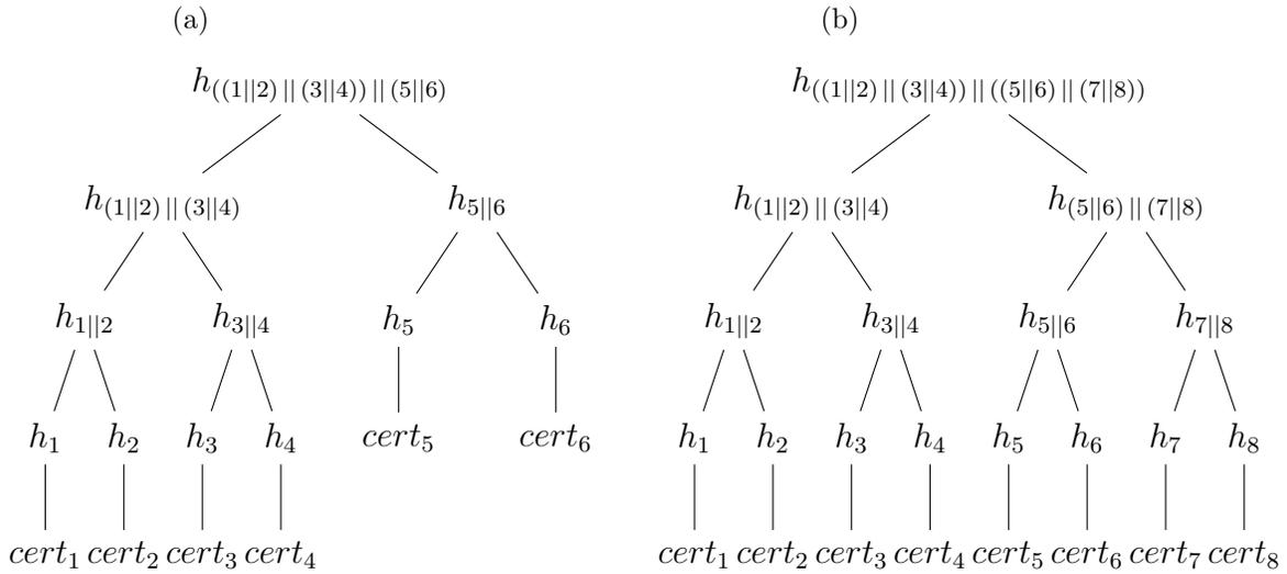
Figure 3.1: A pair of Merkle hash trees with (a) six leaves and (b) eight leaves. Adapted from [42].
