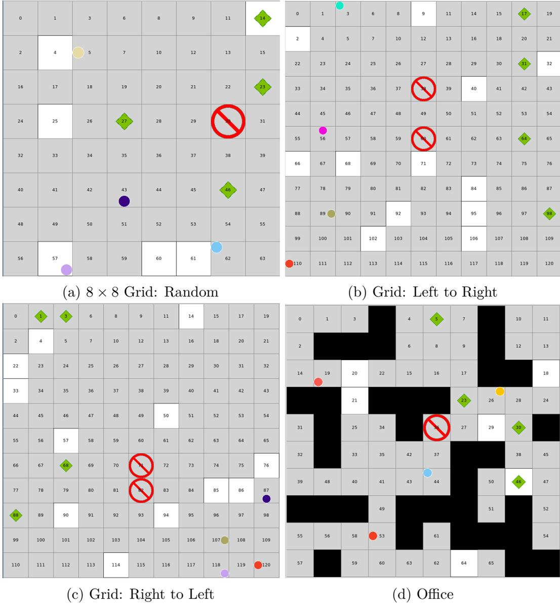
Figure 4.6: Instances of the topological maps used as test environments for benchmarking. Initial locations of robots (4 in these examples) are denoted by coloured circles, task locations are marked by green diamonds and locations to be avoided for the safety specification are shown by a red stop sign. Failure locations ( 90%) are shaded grey.
