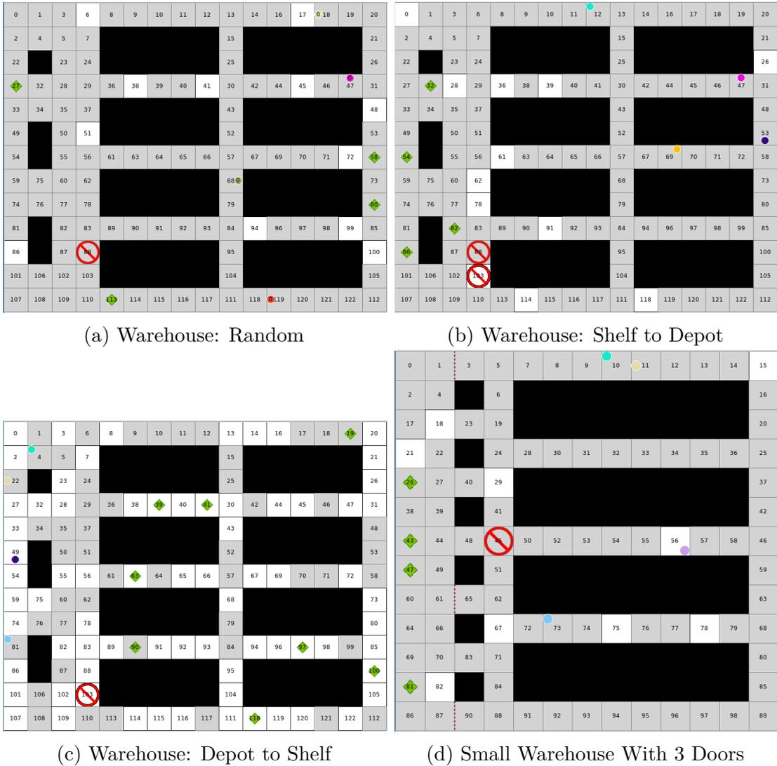
Figure 4.5: Instances of the topological maps used as test environments for benchmarking. Initial locations of robots (4 in these examples) are denoted by coloured circles, task locations are marked by green diamonds and locations to be avoided for the safety specification are shown by a red stop sign. Failure locations (40% of locations in c; 90% elsewhere) are shaded grey. Doors, as used in d, are represented as a dashed brown line between two states.
