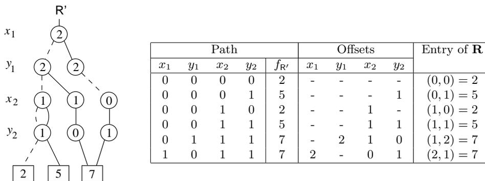
Fig. 6. The offset-labelled MTBDD representing the CTMC in Figure 4
